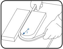
Preheat the heating equipment to 300°F (149°C). Heat light guides approximately 6-15 minutes until soft and pliable. Bend the light guide over a printed pattern, routed template, or use freeforming. A clean flat insulated surface (wood or laminated countertop) will help to prevent twisting or bowing. See the chart above for minimum bend radius guidelines.
