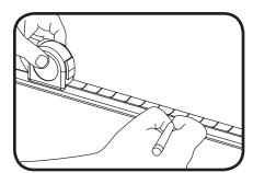
Mark the light guide at the required length, adding 0.5 in. (13mm) for every 16 in. (406mm) to account for shrinkage during the forming process.
