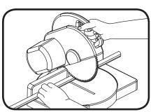
Cut the light guide to the required length using a hacksaw, chop saw (cross cut or veneer blade only), band saw, or other appropriate plastic cutting tool.
