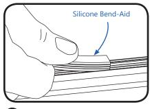
Fill the entire light guide channel with the GEXNBA Silicone Bend-Aid(s) and press into place. Bend-Aid must be installed prior to heating and forming. The GEXNBA Silicone Bend-Aid is reusable.
