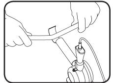
**Part 2:** The workable forming time is about 2–3 minutes. The light guide must remain in the desired position until completely cooled. See the chart above for minimum bend radius guidelines.
