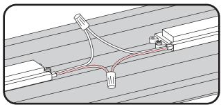
1 Connect modules using twist-on wire connectors or in-line (IDC) connectors. Join white wires together and red striped wires together.
