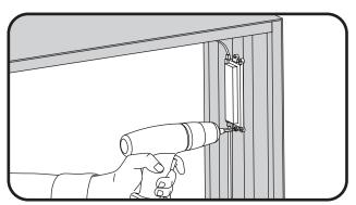
4 Use rivets, screws, or silicone to secure each module within the sign. Use #6 (M3) or #8 (M4) screws, 1/8-inch (3.2 mm) rivets, or silicone.
