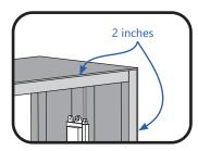
A 2 in. (51 mm) border is recommended along the perimeter of the sign.
