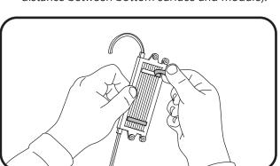
3 Peel off backing to expose adhesive tape and stick LED modules into place.
