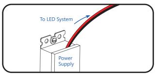
Run a wire from the Power Supply and connect to the first LED module on the strip.
