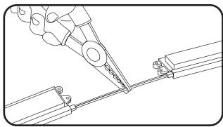
2 Determine how many modules are required for your application and cut where necessary.
