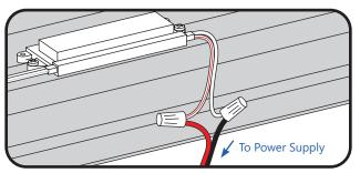
4 Connect the red stripe wire (+) of the LED system to the red wire (+) of the power supply. Connect the white wire (-) of the LED system to the black or blue wire (-) of the power supply.
