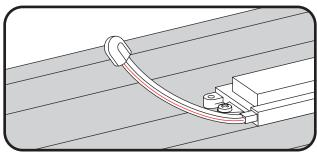
2 Cap all exposed wires with appropriate end caps or apply electric grade (non-conductive) silicone for additional weather protection.
